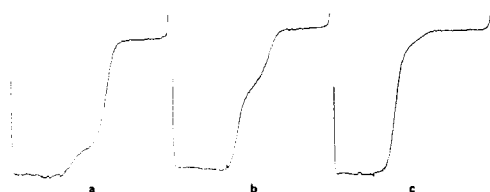
FIGURE 5: Densitometer tracings representing sedimentation patterns of RNA samples extracted from TY-A preparations resulting from alkaline degradations of TYMV (pH 10.35, 30°, 1.0 M KCl) at different lengths of time. Sedimentation from left to right. Pictures taken about 20 min after centrifuge reached speed of 42,040 rpm. Cell, synthetic boundary; a, RNA from TY-A (2 min); b, RNA from TY-A (8 min); c, RNA from TY-A (16 min).
